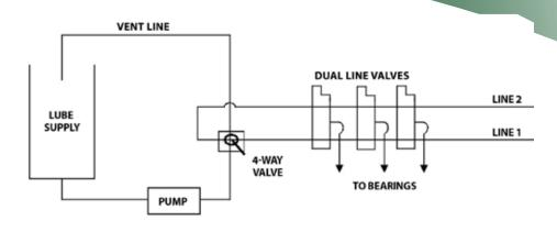
degrees, directing flow through the second line, which supplies lubricant to the bottom inlet of the measuring valve. This type is usually used where long runs or low temperatures are encountered. Points can easily be added.
