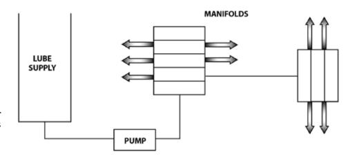
the correct amount of lubricant is delivered to the desired component. This type is typically used where the number of system points are fixed and will not need to be changed
